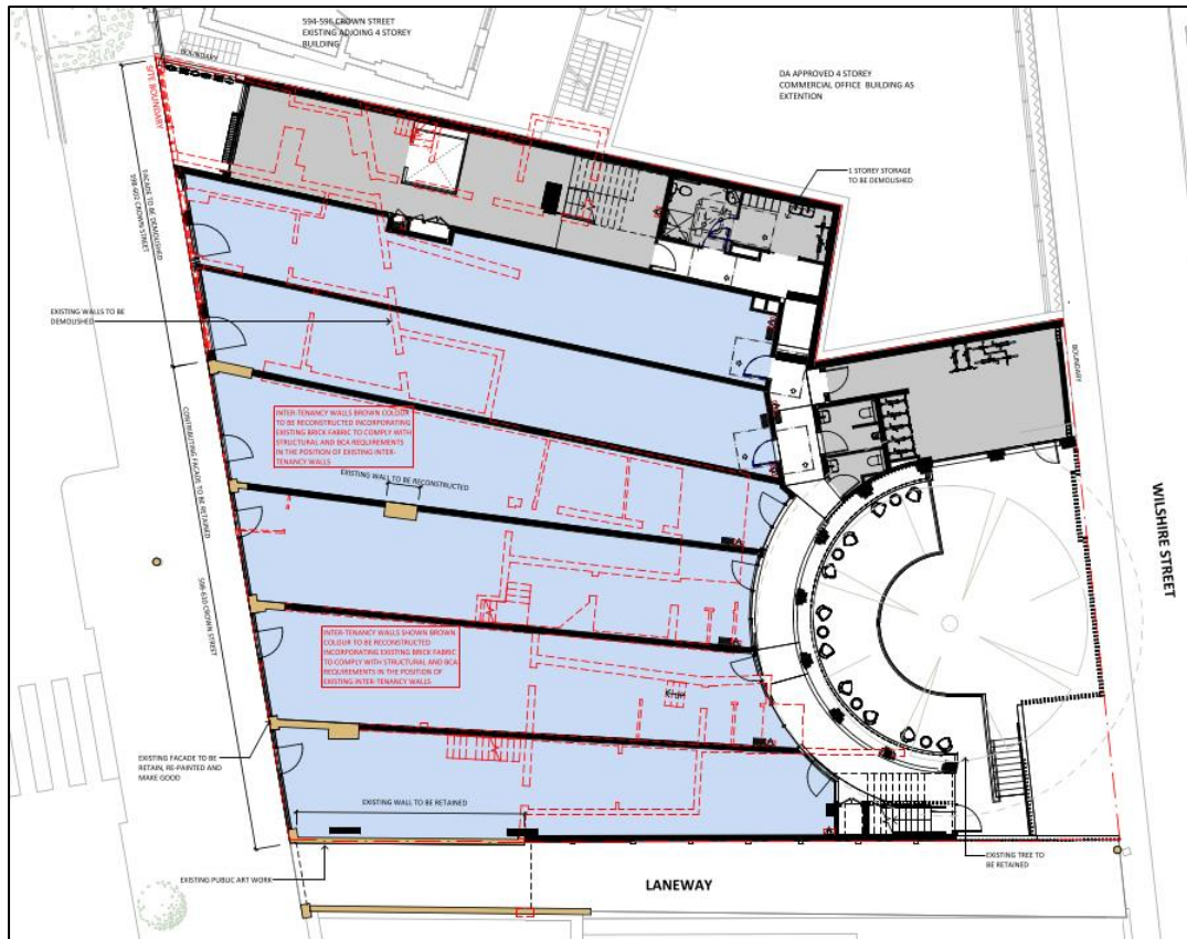
Figure 47: Original DA ground floor demolition plan showing new walls in black and demolished and reconstructed walls in brown
