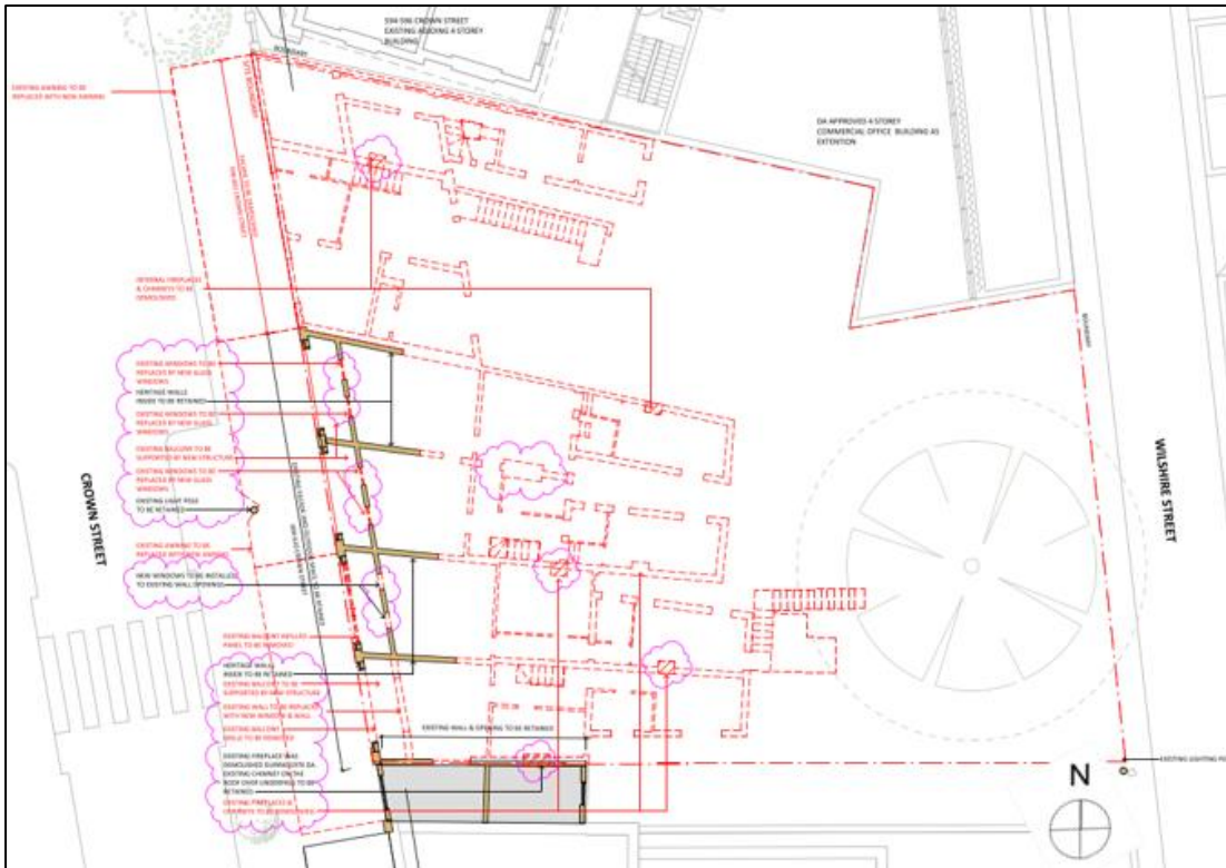
Figure 18: Proposed level 1 demolition plan
