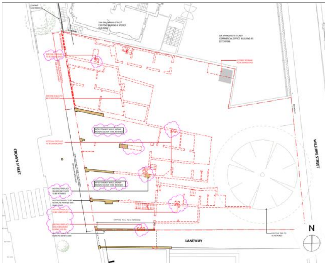
Figure 17: Proposed ground floor demolition plan
